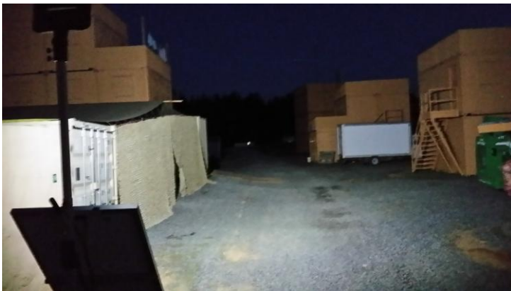
Illumination Pattern of One(1) Portable Solar Powered LED Flood Light Cart Shown Above
